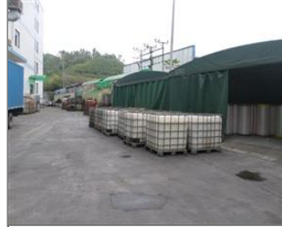
Photo of non-conformity NC5 chemical stored in open area without properly protection.JPG
